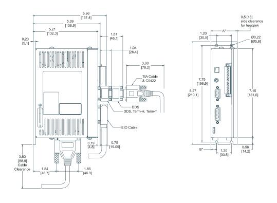
Figure 45: Drive Dimesions Eb-202, Eb-203, Eb-205
